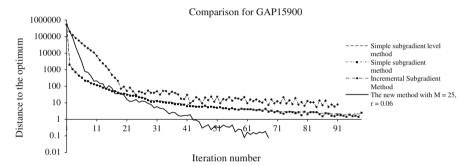
**Fig. 5** Comparison of the surrogate Lagrangian relaxation method with parameters M=25 and r=0.06 against: I the simple subgradient method with  $\alpha=1$ ; 2 the subgradient-level method with parameters  $\delta_0=50000$  and B=750; 3 the incremental subgradient method with parameters  $\delta_0=50000$  and B=750
