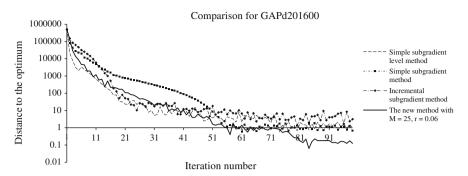
**Fig. 4** Comparison of the surrogate Lagrangian relaxation method with parameters M=25 and r=0.06 against: I the simple subgradient method with  $\alpha=1$ ; 2 the subgradient-level method with  $\delta_0=100000$  and B=500; 3 the incremental subgradient method with parameters  $\delta_0=100000$  and B=1000
