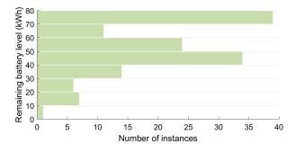
Fig. 7. Distribution of EV remaining battery levels when leaving the charging station in one testing episode.
