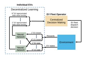
Fig. 1. Overall reinforcement learning framework.
