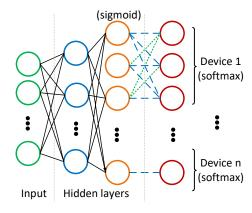
Fig. 1. Device-decoupled structure of the policy neural network
