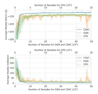
Fig. 2. Average weekly return and voltage violation for 4-bus test feeder
